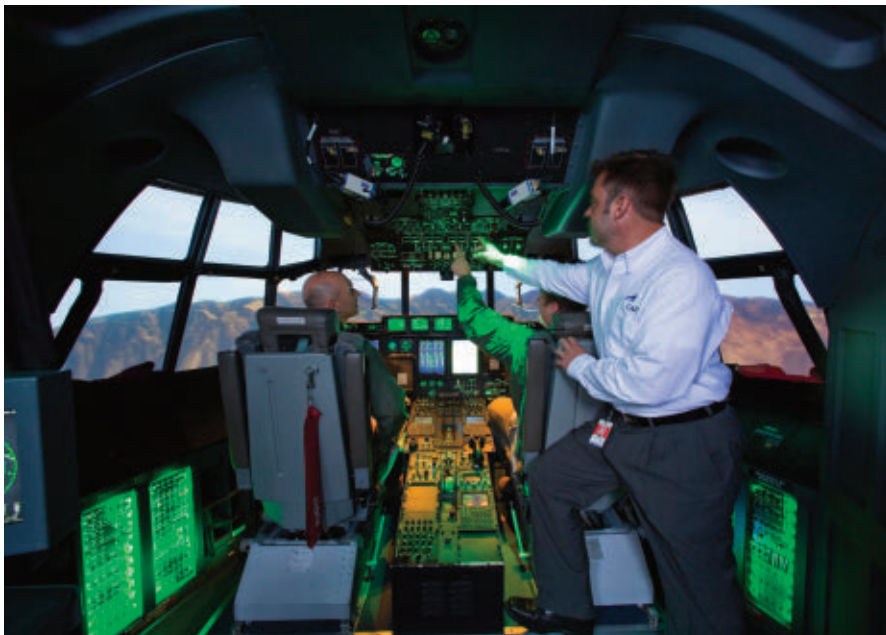
CAE's full-mission simulators, such as the C-130J simulator for the U.S. Air Force above, are helping militaries increasingly use simulation-based training to maintain readiness more cost-effectively.
